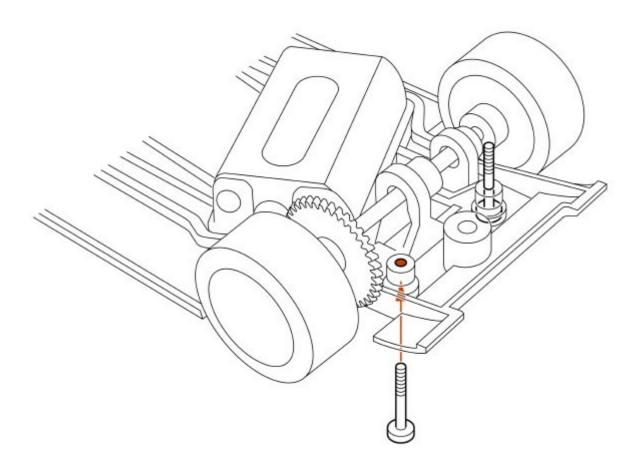
It is now the turn of the photoetched plate. It will be necessary to screw the brass screws through the plate because its holes are very precise. Note please that the plate has thicker circles around the external holes: these are made to keep the spring in place, so make sure they are facing up.
