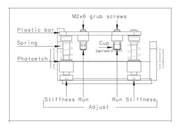
Once assembled inside the car, both the stiffness of the springs and the length of the run of the suspensions can be adjusted without removing the chassis.
