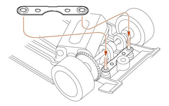
Now it is time to put the spring in place, and to top everything with the plastic bar which was previously assembled.
