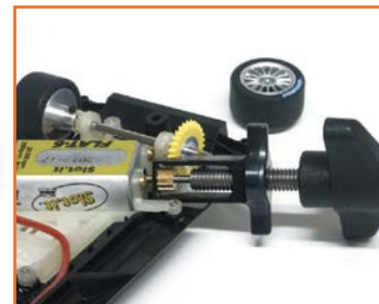
Pull the pinion leaving motor and crown in place
