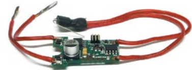
SP15 Universal Hornby SSD upgrade PCB
