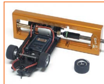
Push the pinion leaving motor and crown in place
