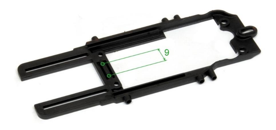
The older HRS2 chassis can be made compatible with the SCX system by drilling two holes 9 mm distant, with a diameter of 1.8 mm.
