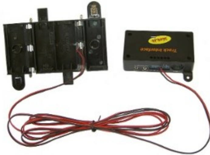
Figure 28: example of the connection of the Track Interface to a dead strip.
