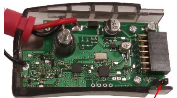
Jumper: remove for SCP 1.1 and 2 leave for SCP 1.0
