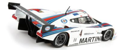
Chassis was made of aluminium and magnesium while body was carbon fibre composite. The overall weight was 850 kg.
