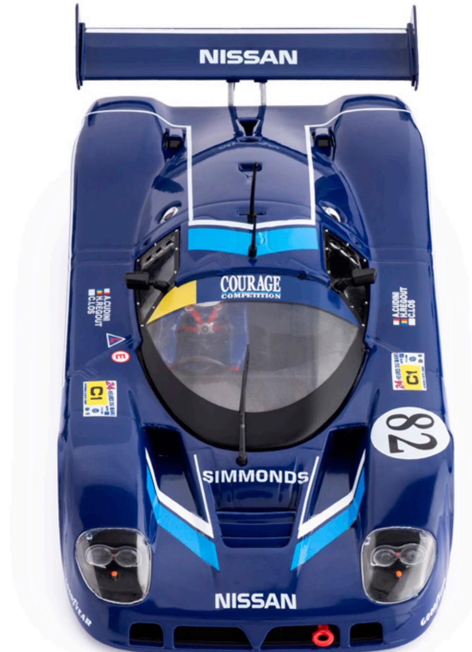
For the 1989 season, rather than relying again on chassis built by March, Nissan had developed the R89C model in conjunction with Lola. The car featured a kevlar and carbon-fibre based monocoque chassis fitted with Nissan's new twin-turbo VRH35 3.5L V8 DOHC engine which was mounted in a stressed installation for better chassis rigidity, delivering up to 950bhp.
