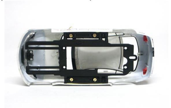
and adjust the overall width of the chassis to the width of the model itself, by setting the 8mm grub screws' position:
