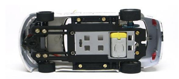
It is now time to assemble the HRS2 chassis with motor pod, wheels, and pickup, and roughly adjust the chassis wheelbase and pickup position to the final specification. What is really important now is to place the rear wheels exactly in the center of the rear wheel arch.
