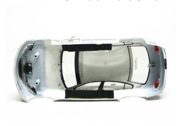
Now, with epoxy resin or other glue of your choice, bond the 'L' shaped bars permanently to the body. Cyan glue is not recommended for this operation as it is quite fragile in case of hard hit on the flexible plastic.
