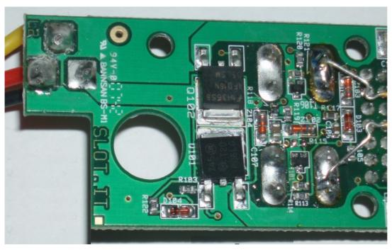
2. Cut the RED line with a cutter's edge, or, remove diode D104
