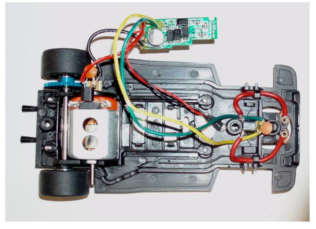
5. Stick the SSD F1 chip behind the cockpit. Solder the SSD power wires to the motor.
