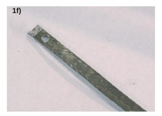
Alternatively, insert the braid inside the pickup and use a small tip to open a hole in the braid, which, being inside the pickup, will retain its shape during drilling.
