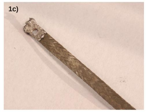
Solder one end of the braid. Leave the solder thin enough to enter inside the pickup Drill a (approx.) 1.5mm hole
