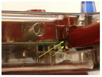
Spray a little in the small hole on top of the screw which keeps the trigger in place:
