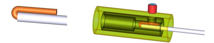
It is recommended to make sure that both the stripped cable, and the platic wire itself, are pressed by the grub screw.
