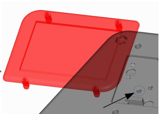
3 - When the support is fully inserted in the hole, it will click and stay there. Insert the support in the hole until it clicks! Now peel off the yellow sticker 'skin'.
