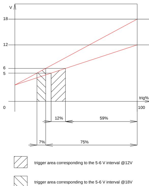
UK Let's suppose in a given turn the car can be driven optimally in a voltage range between, say, 5 and 6 Volt. In the given example (which is an example only), at 12V this range falls across a 12% band, which, in turn, is located approximately 30% from 0. But look at what happens at 18V: the same 5-6 Volt band is now spread across a 7% band, which is also much closer to the 0 position
