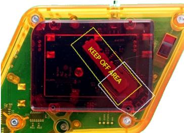
Starting in April, 2022, the SCP-3 radio section has been upgraded, incorporating a 3dbm gain antenna, to improve the radio range of the controller. The SCP-3 rel. B can be identified by looking at the back side of the case: the antenna, and underlying 2.4GHz module, are found inside the yellow and white dotted lines, respectively.
