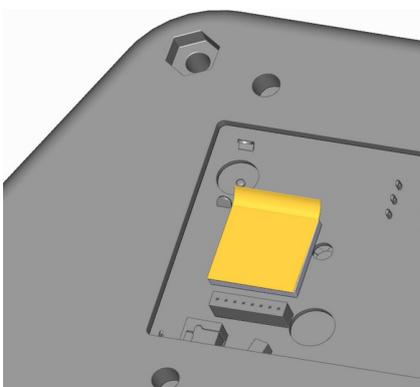
4 - Now it's time to insert the module into place. The module is connected with eight pins that must match the eight holes on the female connector. Make sure that the male pins on the module are aligned to the 8 holes in the receptacle:
