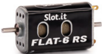
MN14H Flat-6RS 25.000 rpm - 240g*cm @12V - asymmetric case openings
