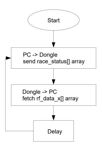
The 'delay' value is strictly connected to the speed of the PC speed and its tasks' load, and this in turn may affect the speed of the RMS. Note that each controller sends its data back to the dongle with a 600ms cycle time (i.e. every 600 ms).
