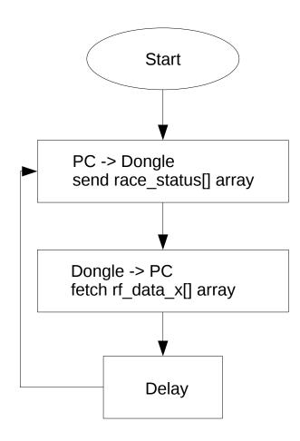
The 'delay' value is intricately linked to the speed of the PC and the workload it is handling, which consequently impacts the performance of the RMS.
