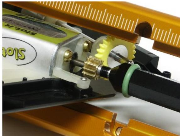
7. Press the pinion in place and remove tool. Done!
