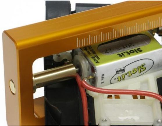
6. Place the pinion on the retractile pin (spring actuated) and adjust distance to bring the pinion and the shaft in contact. Now make sure the pinion is properly aligned with the shaft.
